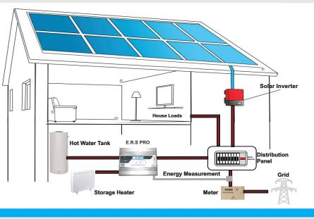
Typical system layout: Other configurations are possible
