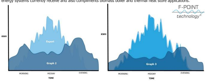
Graphs 2 and 3 above show a comparison of a solar system with and without ERS. The light blue in graph 2 highlights the export that occurs during the day. Graph 3 shows how ERS tracks the export and recovers it without suffering from the 'tail off' resulting in imported energy during the operation as compared to graph 1.
